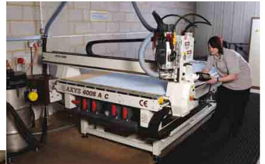
CNC machine for routing panels and worktops
