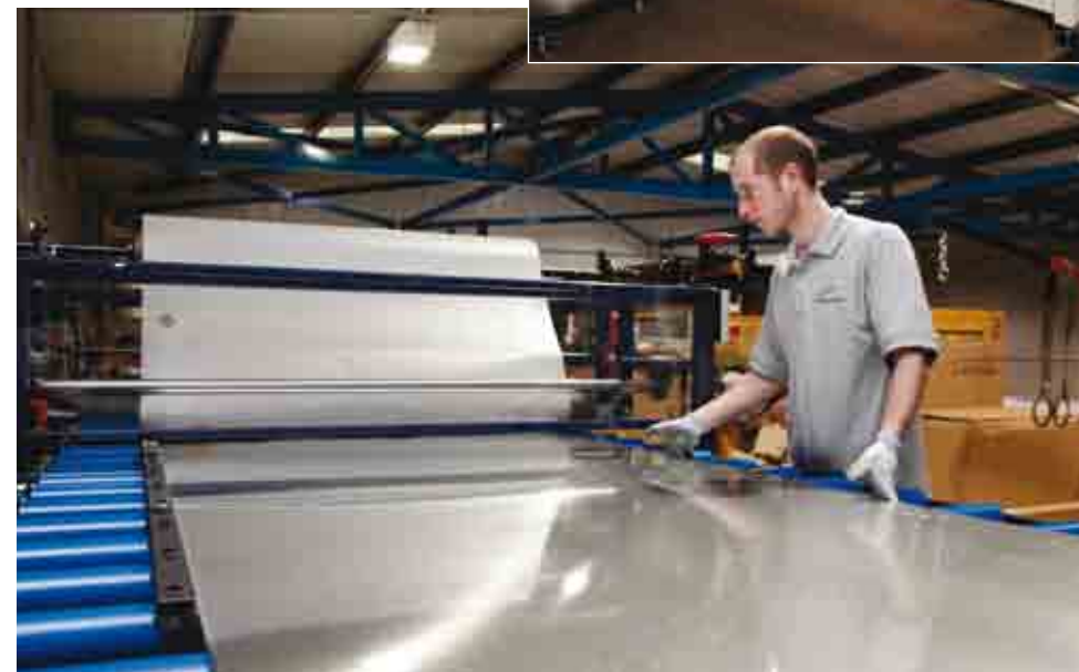
All cladding material is laminated in-house
